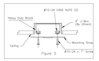
Complete the installation in accordance with the fixture installation instructions, attaching the fixture mounting strap to the Heavy Duty Brace with the #10-24 machine screws provided. See Figure 3.
