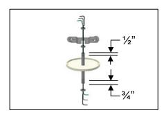
2b. At feed location - Securely fasten the mounting strap on to the stem at the 1/2" end. Place the stem through the canopy. Thread one nut on the other end of the stem. Insert the power wires wires through stem.
