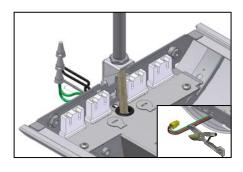
7b. At feed location - Insert power wires through sleeve, bushing, and knockout on the male connector end of the fixture. Hook stem hanger onto fixture. Secure the hanger with #8 flat head screw. Cut off male wire connector. Install end-cap.
