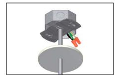
4b. At feed location - Splice the fixture power wires and building power wires together in the junction box. Raise the canopy in to place.
