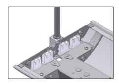
7a. Non-feed location - Hook the hanger to the female connector end of the fixture. Cap unused wires where applicable. Install end-cap.
