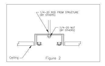
Determine the appropriate support method for ceiling construction (sample method is shown on Figure 2). Attach the appropriate fastening devices through the holes of the bracket and box and secure the assembly to the support structure.
