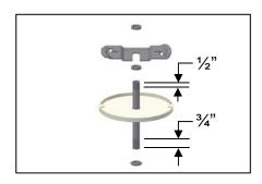
2a. Non-feed location - Securely fasten the mounting strap on to the stem at the 1/2" end. Place the stem through the canopy. Thread one nut on the other end of the stem.
