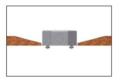
1. Secure the 4" octagonal junction box so that it is flush with ceiling level.
