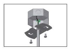
Raise stem set in position. Install the mounting strap to the junction box with two screws. See page 3 & 4 of this installation if using heavy-duty brace.
