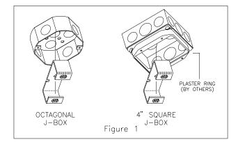
Insert the Heavy Duty Brace diagonally into the J-Box and align the holes in the bracket with the existing holes in the J-Box.
