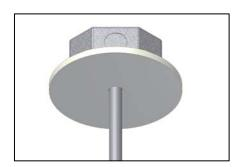
Twist the canopy clockwise onto the mounting strap securely to complete the installation.
