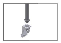
Insert the stem at 3/4" end onto stem hanger and lock with bottom and top nuts.
